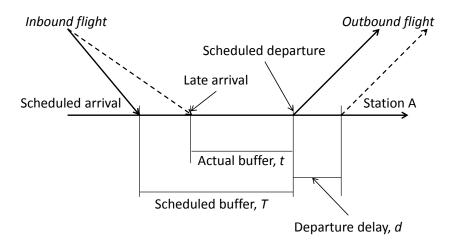
Figure 4: Flight sequence within an aircraft rotation depicting scheduled and actual ground-time buffers.
